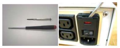
2. Using the smaller screwdriver slightly pull the fuse holder out
