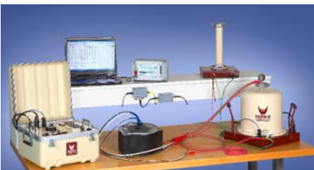
Partial Discharge Test Setup used by Powertronix to Test Insulation Quality
