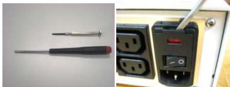
2. Using the smaller screwdriver slightly pull the fuse holder out
